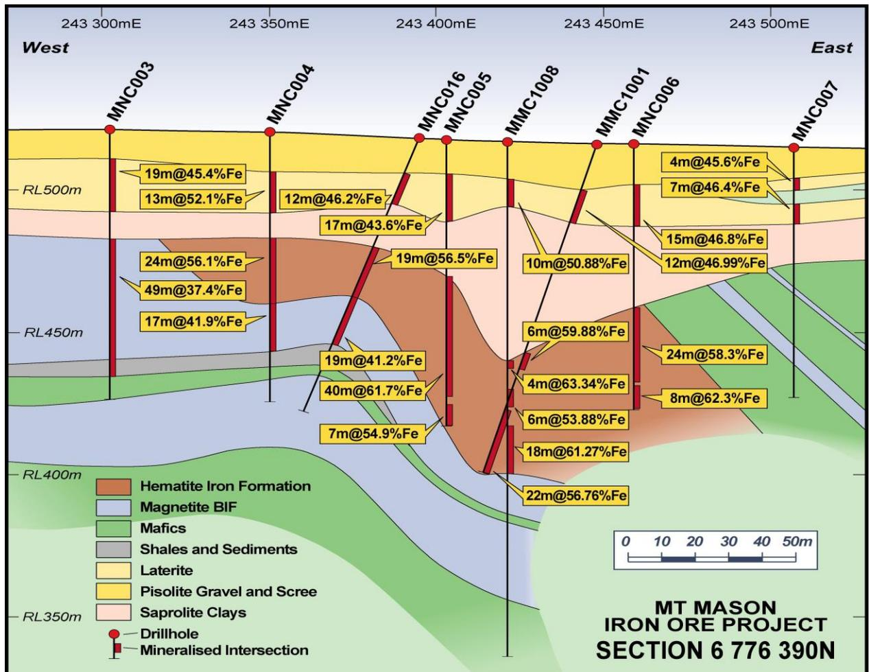
**Figure 3: RC Drilling Program – Drilling Cross Section 6 776 390N.**
