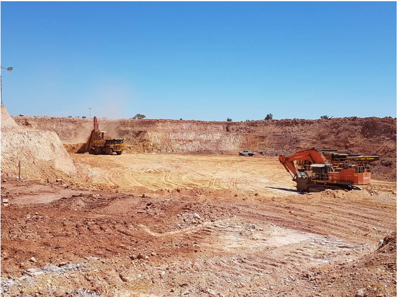
Figure 1. Mining at the Trouser Legs JV Gold Project – 2 x 120 Tonne Excavators, 4 x Cat 777 Dump Trucks in Pit
